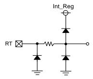
**Equivalent Circuit for RT Pin**
