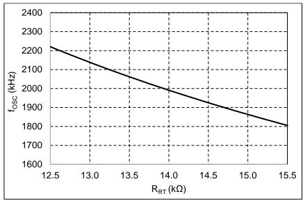
$R_{RT} [k\Omega] = 37773 \times f_{OSC} [kHz] \wedge (-1.04)$ R1275S Oscillator Frequency vs Oscillator Frequency Setting Resistance
