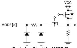
Equivalent Circuit for MODE Pin
