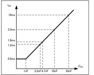
$$\begin{split} &C_{\text{SS}}\left[\text{nF}\right] = (t_{\text{SS}} - t_{\text{VO}\_S}) \ / \ 0.64 \ \times \ 2.0 \\ &t_{\text{SS}}: \ \text{Soft-start time} \ (\text{ms}) \\ &t_{\text{VO}\_S}: \ \text{Time period from} \\ & CE = \text{``High'' to VOUT's rising} \\ & (\text{Typ. 0.160 ms}) \end{split}$$
