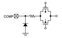
Equivalent Circuit for COMP Pin
