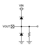
**Equivalent Circuit for VOUT Pin**
