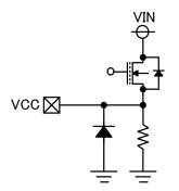
**Equivalent Circuit for VCC Pin**
